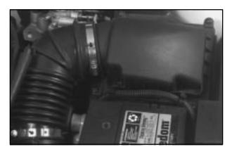
The air cleaner is located on the driver's side of the engine compartment near the battery.
